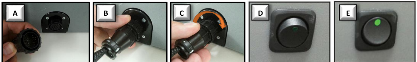
Figure 2A through 2E. Connecting your welding gun and powering-on the equipment
