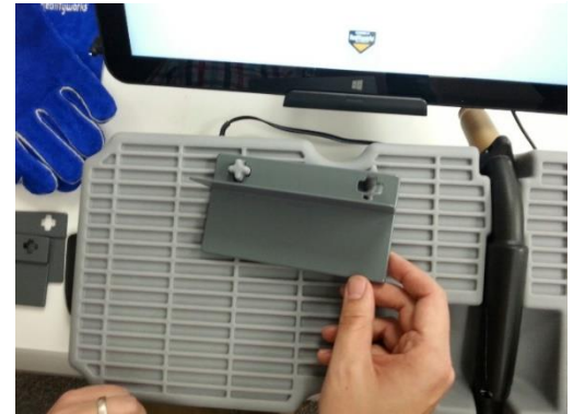
Figure 25. Placing the coupon on the workstation
